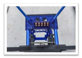
The final step in the frame assembly is the installation of the *LED Board* (A) and the Antenna tubes into the **Receiver, VTX, LED and Antenna Tray** (K).
