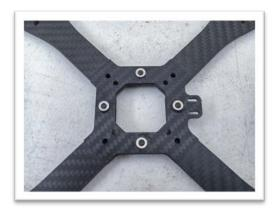
We can now remove the **M3 X 14mm bolts** (J) that where temporarily used to keep the sandwich together, they will be used later to mount the battery plate and the standoffs. The pictures above show what the main frame sandwich should look like from the bottom and from the top when completely assembled.
