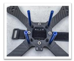
The battery strap can now be permanently installed. It is held in place using the *Battery Plate* (C) and *the M3 X 14mm Bolts* (J). The battery plate bolts will screw into the *4omm Standoffs* (C). This is another place where you can use thread-locking compound if desired.
