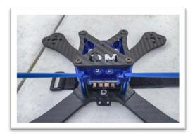
Once the receiver plate and the camera assembly have been installed you can install the *Top Plate* (D) using the *M<sub>3</sub> X*\*\*8mm Bolts\* (H). The cutout in the top plate faces the front of the frame.
