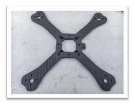
Place the *4mm Arms* (E) over the *M3 X 14mm bolts* (J), this will ensure that they are in the proper location. The arms should come together at the inside edges and the semi-circular notches will line up with the press-nuts that are in the main plate.
