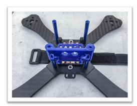
Slide the *Receiver*, *VTX*, *LED* and *Antenna Tray* (K) over the two rear standoffs (the ones closes to the power lead stress relief tab). This piece will hold all the listed components:
