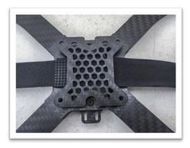
The orientation of the battery strap and the **Battery Plate** (C) must align with the orientation of the **Bottom Plate** (B).
