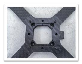
Place the *Bottom Plate* (B) onto the assembly as shown in the picture to the left. Please note the orientation of the opening on the bottom plate, the narrow dimension needs to go front to back (please note that this is depicted left to right in the picture to the left as the frame is turned 90° and the battery lead stress relief tab denotes the rear of the frame) and the wider dimension
