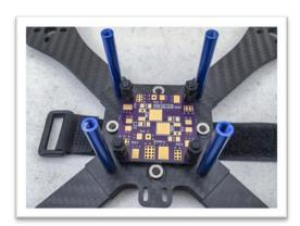
If you did not install your electronics in Step 1 above then you can install them here. The *PDB* (B) is held down by the *Nylon*Standoffs (D) and the flight controller board is held down by the final set of *Nylon*Nuts (D).
