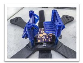
Prepare the camera assembly off the quad before installing it. The camera mounts to the *Camera Plate* (L) using the provided *M2 X 8mm* (F) bolts. The camera installs from the rear (the side that is not smooth) and the bottom of the camera aligns with the narrow side of the *Camera Plate* (L) (the side with the rounded corners).
