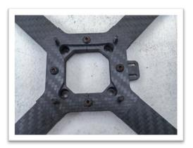
At this point in time the mainframe sandwich can be completed by using the main sandwich *M3 X 10mm bolts* (I). Align the arms properly, insert and screw in the main sandwich bolts loosely until all 4 are in place. If you use thread locker on your frames now is the time to apply it to these bolts. Once all four bolts are in position then they can be tightened down to complete the main frame sandwich.
