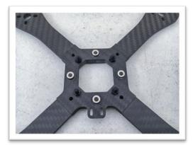
Start the stack assembly by installing the *Nylon Bolts* (D) through the inside holes in the corners. The bolts are held in place with a nylon nut as shown in the picture to the left.
